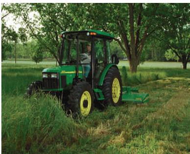
Personnel should stay clear of rotating drivelines. Never try to remove debris or get close to the machine blades without making sure the mower is fully shut off and all shut down procedures have been followed.
